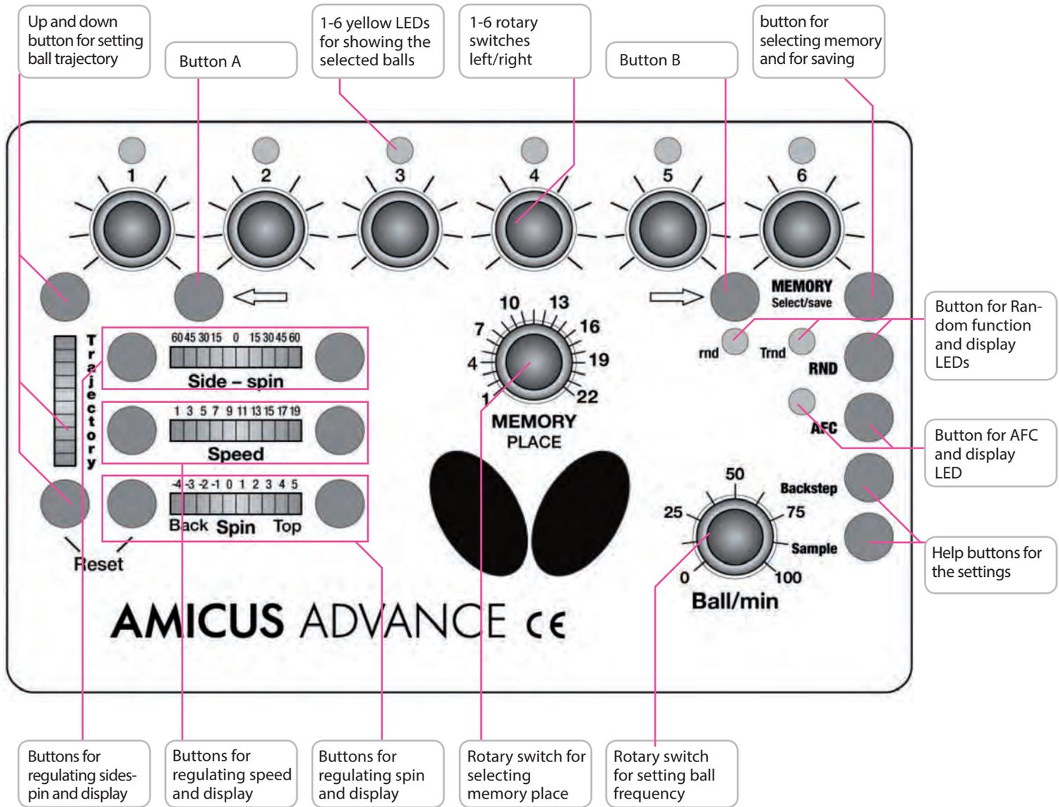
With the help of rotary switches 1-6 above and the buttons, it is possible to program six different landing spots, for example Ball 1 \* middle, Ball 2 \* left, Ball 3 \* right, Ball 4 \* right ... See illustration.
